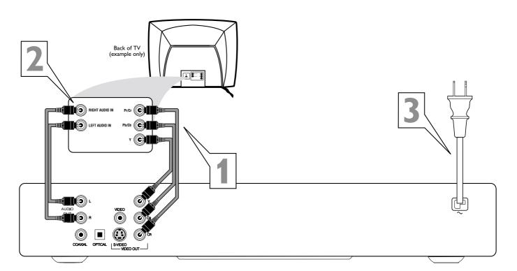
Connect the DVD Player's Y CB CR (VIDEO OUT) jacks to the corresponding COMPONENT VIDEO IN jacks on the TV. Use component video cable (not supplied).
